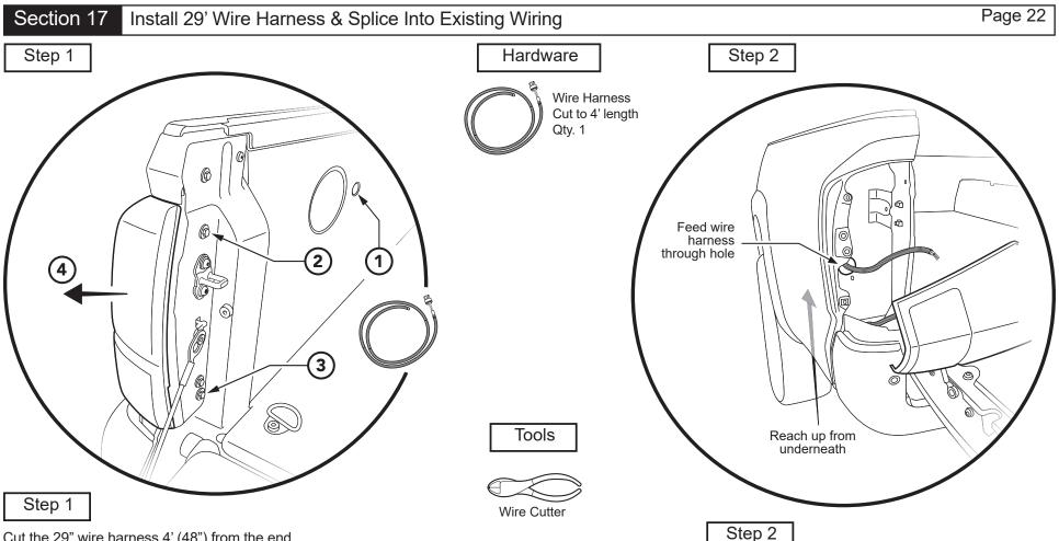
Cut the 29" wire harness 4' (48") from the end with the connector. Feed the cut end through the side of the bed at location (1) and through the slot underneath the edge of the cap. Leave about 5" of the wire harness with the connector inside the vehicle bed.
