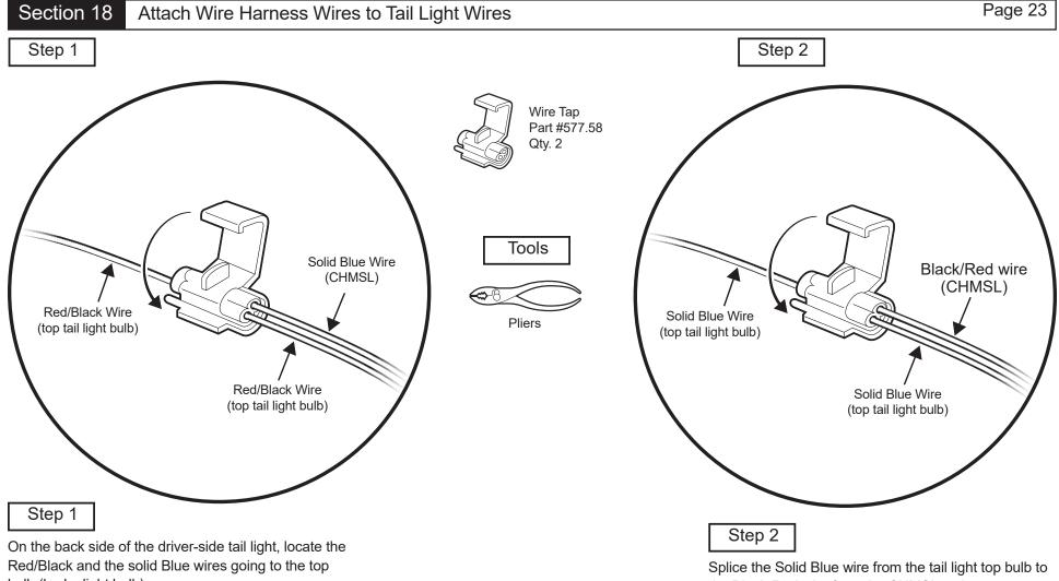
bulb (brake light bulb). Splice the Red/Black wire from the tail light top bulb to the solid Blue wire from the CHMSL, using
